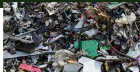
Fluff from separated fraction / Fluff da frazione deferrizzata
